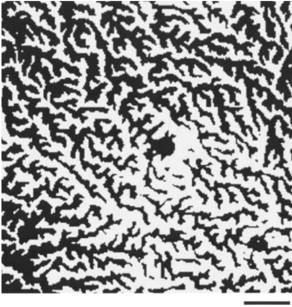
Fig. 7 Patterns formed for CS-82 spheres on a cover glass at 25 °C. In water, \phi = 1.33 \times 10^{-3} , 0.1 ml, length of the bar is 20 \mu\text{m}
